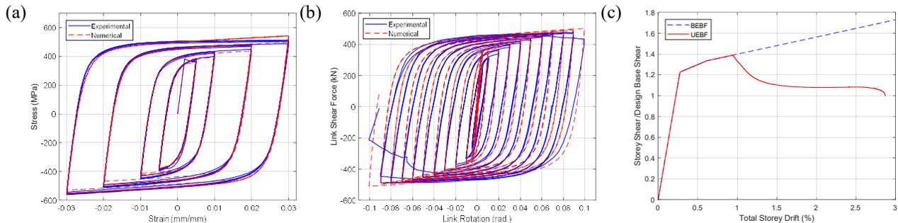
Figure 4. (a) Calibration of Giuffrè-Menegotto-Pinto material model (data by Dehghani et al. 2016 [18]); (b) Shear force-shear deformation behaviour of the W250x28 link (data by Okazaki et al. [21]); (c) Lateral force-lateral deformation response.
