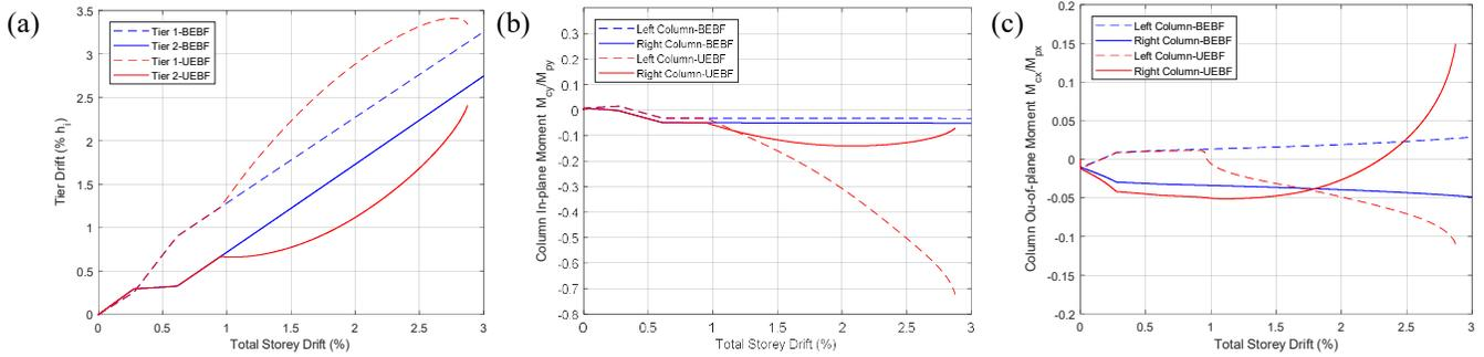
Figure 5. (a) Tier drifts; (b) Column in-plane bending moments; and (c) Column out-of-plane bending moments.
