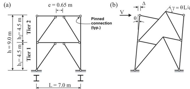
Figure 2. (a) Geometry of the selected two-tiered EBF; (b) Expected plastic mechanism of two-tiered EBF with shear links under seismic loads,  $\theta$  = tier plastic rotation  $\Delta$  = tier lateral deflection (deformations and rotations shown for Tier 2 only).
