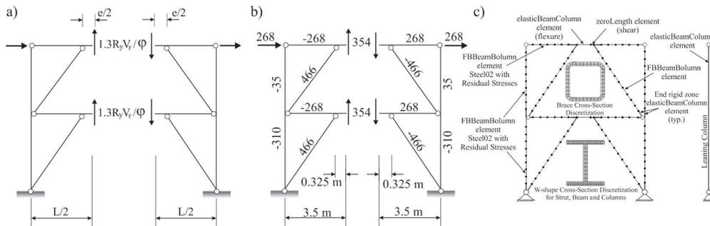
Figure 3. (a) Probable link resistances; (b) Capacity-induced seismic forces under the probable link resistance (forces in kN); and (c) Numerical model of the two-tiered eccentrically braced frame.
